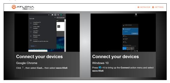
The landing page will provide quick instructions for connecting to the WAVE-101 for casting. This page will display instructions based on the type of device connected. **e.g.** When a Windows OS device is connected it will display instructions for Miracast and, if connecting to the WAVE-101 using a Chrome browser, Chrome cast.
