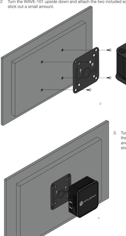
3. Turn the WAVE-101 so that the screws line up with the large oblong shaped holes on the VESA mount and mount the unit to the mounting plate. The unit should slide down if fully on the VESA mount.
